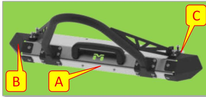
Mid-Stinger Support Flanges(C) will mount on top of Bumper Cap and align with the same three holes. Mid-Stinger Support Flanges use the ½” Oversize Washers provided.
