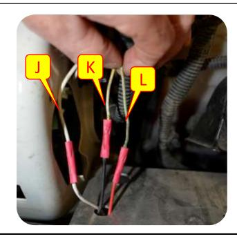
**Note:** Use Electrical Tape or Zip-ties to stow the wires and protect any open connectors.
