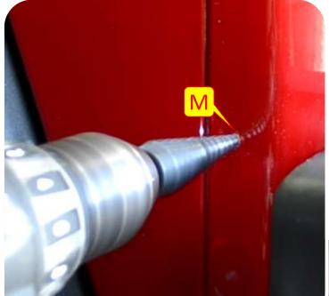
**Note:** We use a step drill after this to chamfer the edges.
