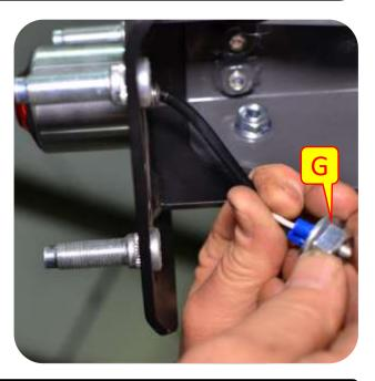
**Important Note:** MetalCloak provides extra wire and splice connectors for swing out tire carriers. If you do not have a swing out tire carrier the extra wire will not be needed.
