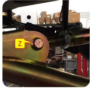
**Note:** To unlock for off-road use, loosen jam nut and spin Lock-N-Load adjuster until corresponding line shows unlocked; Tighten jam nut and go wheeling.
