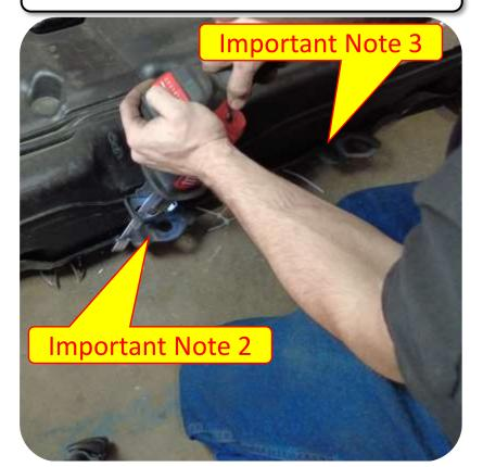
*Important Note 3:* Cut off the rear tab on the gas tank mount next to the one you removed in note 2 as shown. Make sure there is plenty of ventilation before cutting the mount off.
