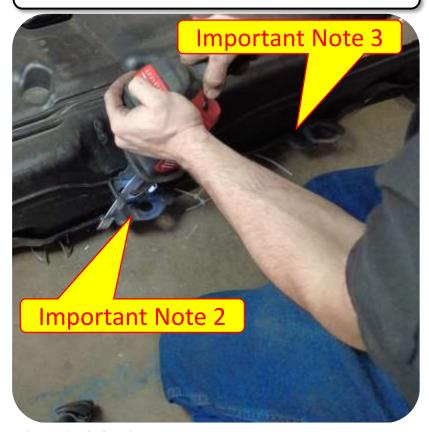
Important Note 3: Cut off the rear tab on the gas tank mount next to the one you removed in note 2 as shown. Make sure there is plenty of ventilation before cutting the mount off.
