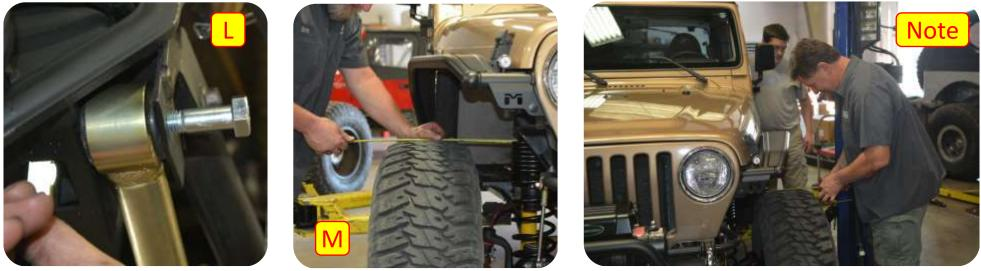
**Note:** Having a second person to turn the steering wheel while centering the vehicle over the axle is very useful.
