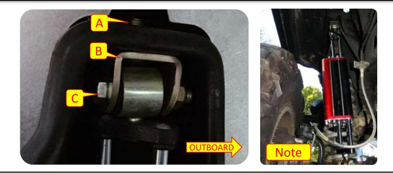
Note: The red reservoir tubes should be oriented toward the rear of the vehicle.
