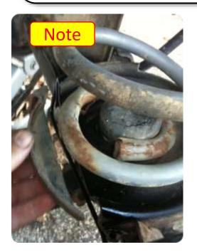
**Note:** For added clearance, trim the stock coil bucket so that it is flush with the rear of the axle. Paint exposed metal.
