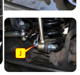
**Note:** The threaded section of rod is not for adjusting the rod length!
