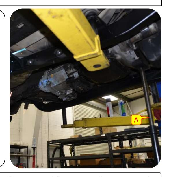
**Note:** The "Rubicon" model TJ's will require relocation of the compressor. The factory compressor bracket may be reused by drilling a hole and mounting it to the seat belt bolt on the underside of the vehicle.
