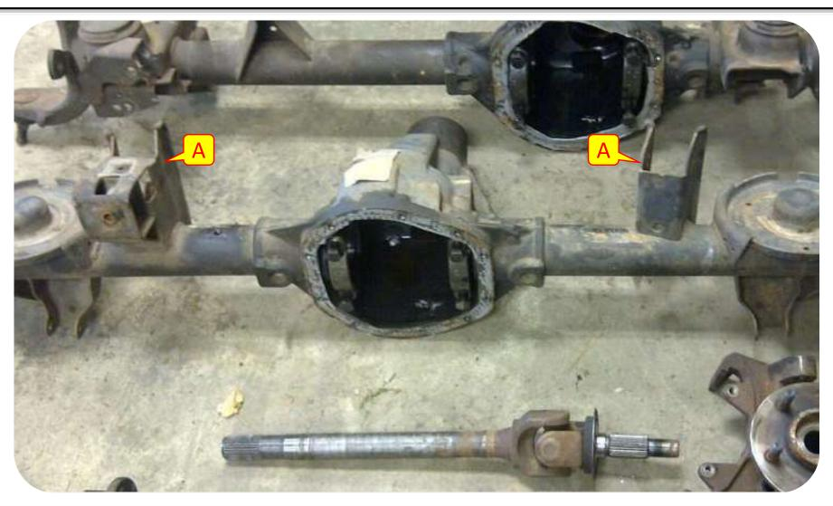
**IMPORTANT NOTE:** THE LOWER BRACKETS REMAIN ON THE AXLE! DO NOT REMOVE THE LOWER BRACKETS!
