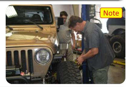
**Note:** Having a second person to turn the steering wheel while centering the vehicle over the axle is very useful.
