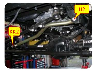
**Note:** It is helpful to have someone push the vehicle to the driver or passenger side to help align the hole; if you don't have an extra pair of hands, you can use a ratchet strap on the frame/axle to pull the frame in the desired direction. Check to ensure the axle is centered once the bolt is in place. If not then remove the bolt, adjust the Track Bar length, replace the bolt, and recheck axle centeredness. Repeat until the axle is as close to center.
