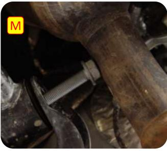
Use the chart below to identify and pre-set the length of your control arms. Hand tighten the lock nuts, for now.
