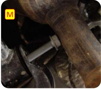
Use the chart below to identify and pre-set the length of your control arms. Hand tighten the lock nuts, for now.
