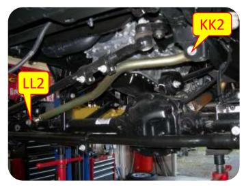
**Note:** It is helpful to have someone push the vehicle to the driver or passenger side to help align the hole; if you don't have an extra pair of hands, you can use a ratchet strap on the frame/axle to pull the frame in the desired direction. Check to ensure the axle is centered once the bolt is in place. If not then remove the bolt, adjust the Track Bar length, replace the bolt, and re-check axle centeredness. Repeat until the axle is as close to center.
