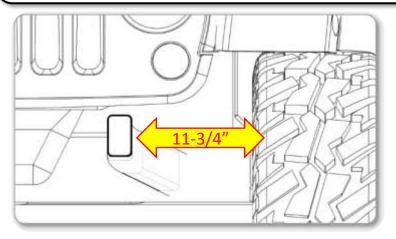
Important Note: To prevent tires from rubbing the shocks at full turn and flex, a clearance of 11-3/4" between inner wall of the tire and the outside of the frame rail is recommended. Wheel backspacing, wheel spacers, axle width and tire width can effect this value. We recommend a wheel backspacing of less than or equal to 4.0" for most common vehicle builds.
