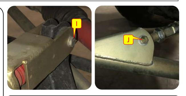
**Note:** To unlock for off-road use loosen jam nut and spin Lock-N-Load adjuster until corresponding line shows unlocked; Tighten jam nut and go wheeling.
