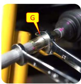
**Important Note:** It's recommended to get your alignment checked after installing the MC tie-rod sleeve.
